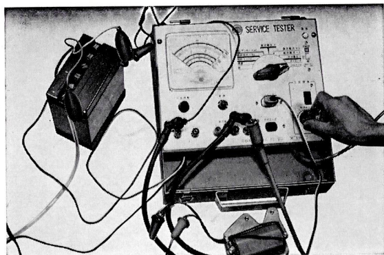
Fig. 5.109 Coil test connection
