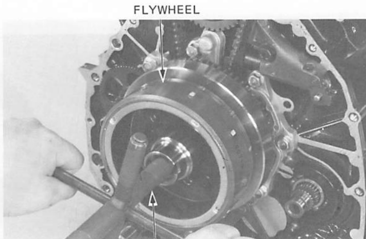
FLYWHEEL PULLER, 20 mm 07933-3950000 OR 07733-0020001
