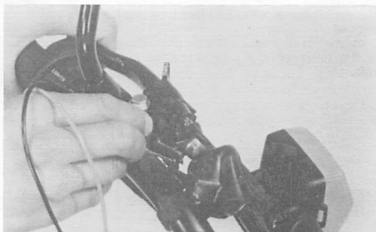
(2) CLUTCH APPLIED: CONTINUITY (3) CLUTCH RELEASED: NO CONTINUITY
